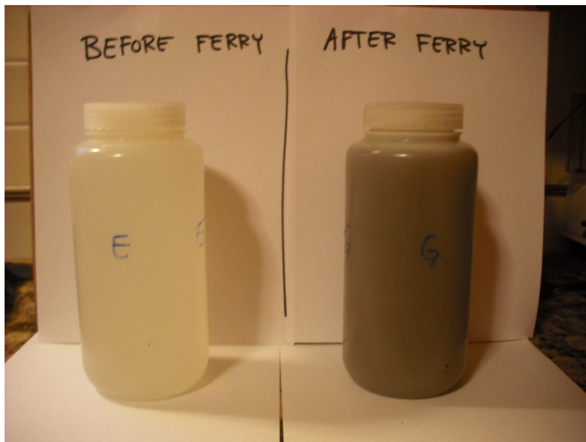
Figure 7. Water samples taken along the shoreline immediately before and after passage of the ferry during low tide (Site 3).
