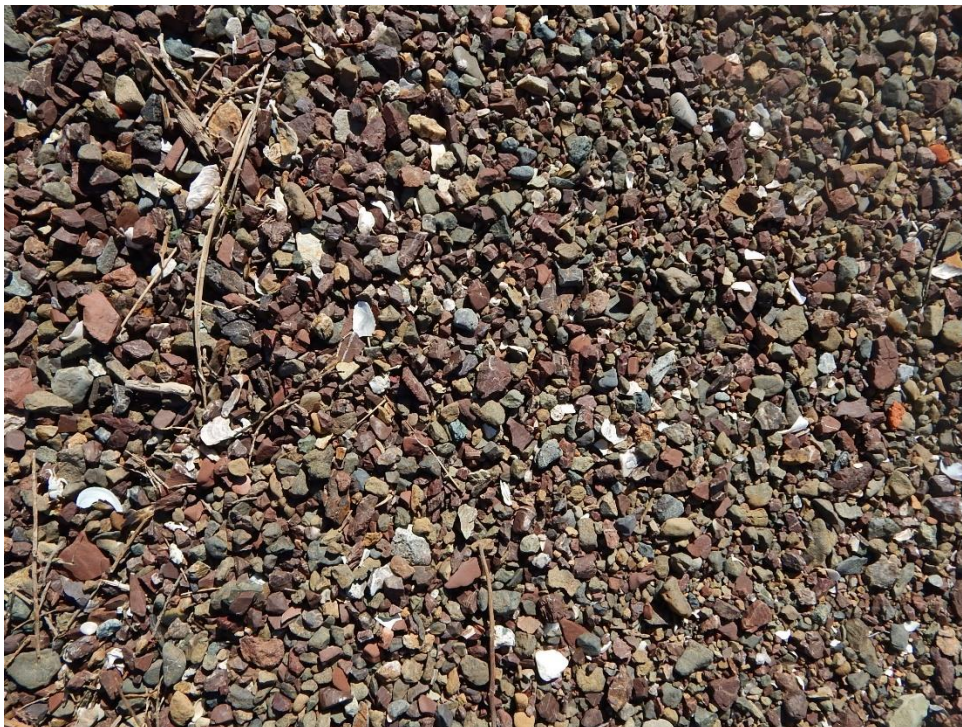
Angular chert (predominant) gravel of berm top and beachface. Matches local Coyote Hills Franciscan outcrops near quarry. Lack of abrasion-rounded or polished sediment indicates origin other than stream gravel or remobilization old beach deposit; no headland sources for angular colluvium.
